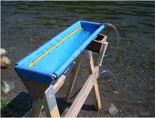
FIGURE 2 Water-filled padded fish sampling trough. The head of the fish is placed at the end with water inflow from a pump to ensure that oxygen levels remain high throughout the sampling event. A measuring tape has been integrated into the trough to simplify processing (Photo credit: Steven Cooke)
